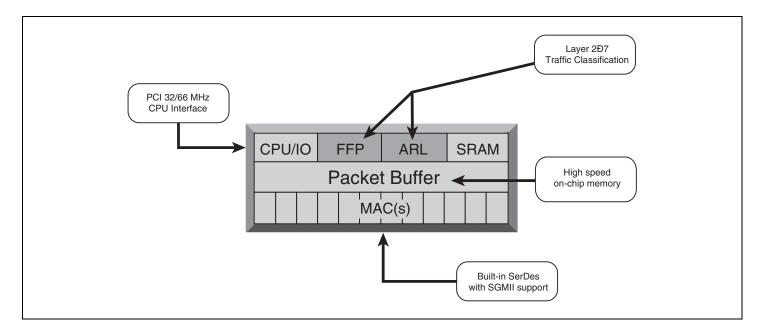
The BCM5691 network switch is a scalable, modular chip solution with 12 ports. Each of these flexible ports supports Gigabit Ethernet or 10/100 Mbps Ethernet. Additionally, the BCM5691 supports both copper and fiber physical interfaces. The BCM5691 has a fully integrated SerDes functionality consisting of a Gigabit Ethernet or a SGMII PHY interface.
