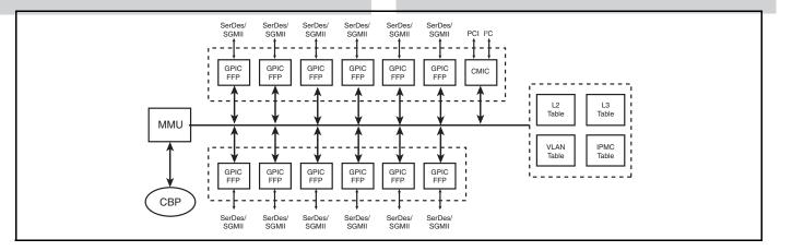
12-Port Gigabit Ethernet Multilayer Switch
